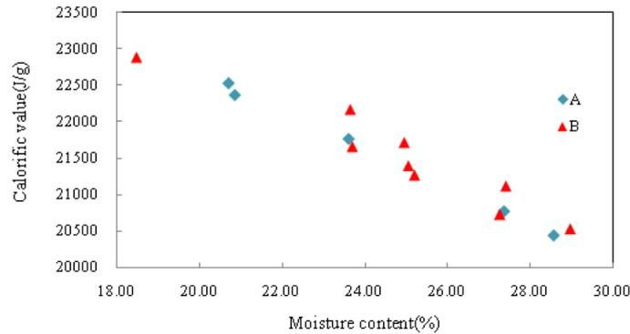
Figure 3 Relationship of calorific value versus moisture content
