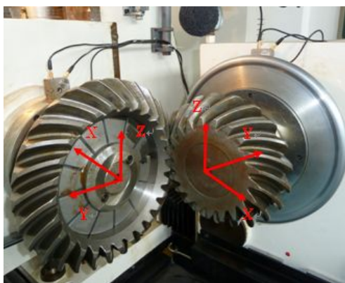
Figure 4 Performance testing of spiral bevel gear mesh experiment
