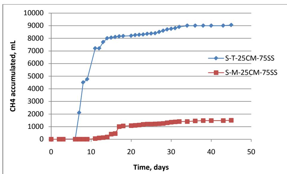
Figure 4 CH<sub>4</sub> accumulated for mesophilic (S-M-25CM-75SS) and thermophilic (S-T-25CM-75SS) tests
