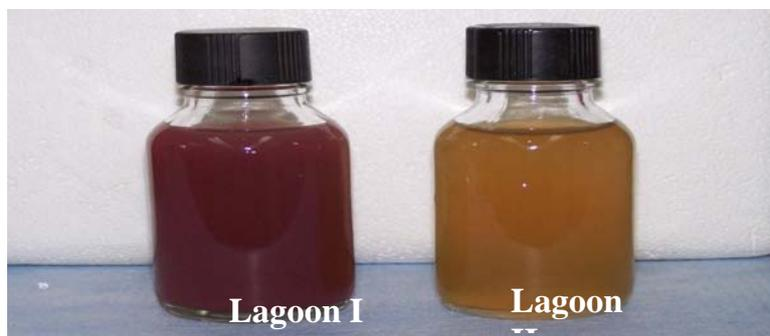
Figure 2 Physical appearance of water from Lagoon I (left; primary treatment system) and Lagoon II (right; secondary treatment system) Lagoon I water was purple and more turbid as compared to water from Lagoon II (see text) which was less turbid and yellowish in color.
