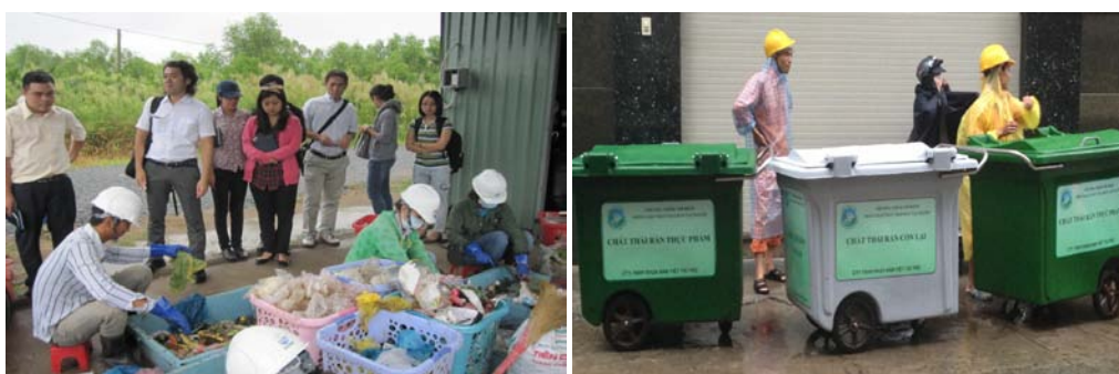
Fig. 1 Collecting and characterizing the composition and quantity of separated waste components from households
