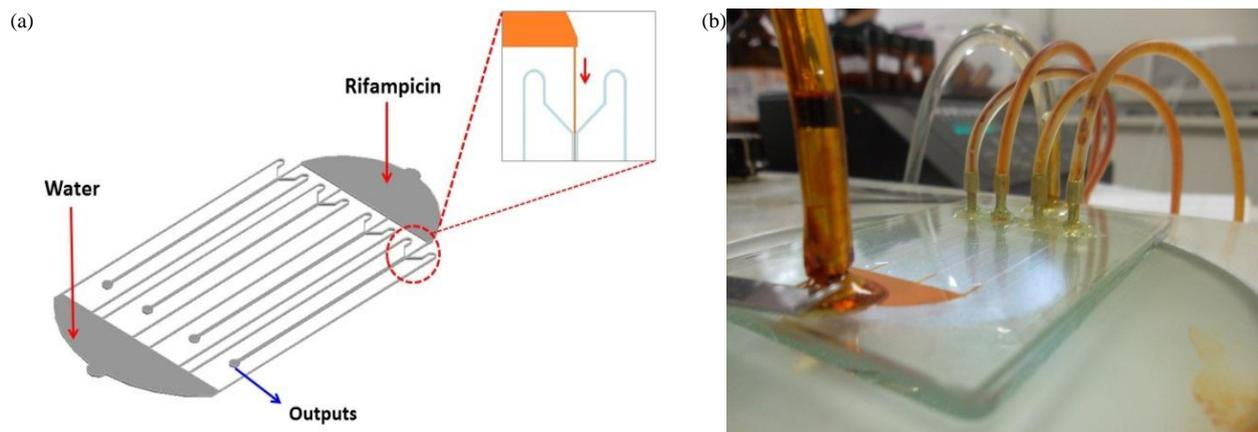
Fig. 1 Parallel microfluidic device with flows distribution by reservoirs: (a) scheme presenting the position of water and rifampicin reservoirs and (b) the microfluidic device microfabricated in glass in operation
