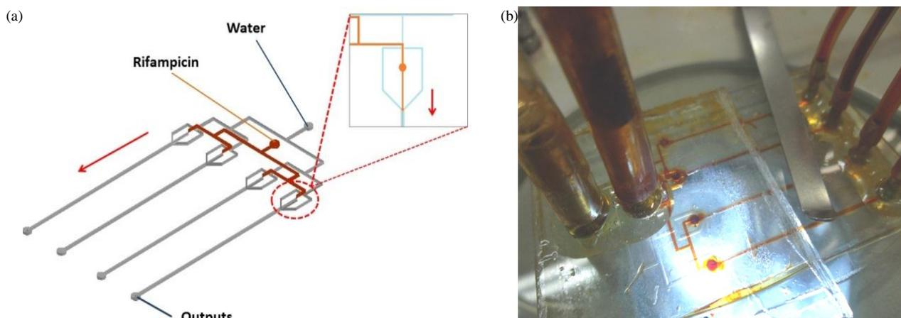
Fig. 2 Parallel microfluidic device with flows distribution by channels branching: (a) scheme of the device that follow the Murrays Law. This device was microfabricated with three glass layers and (b) the device in operation
