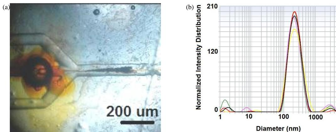
Fig. 6 Rifampicin flow focusing in branch microfluidic system: (a) detail of a flow focusing on using ratio (R) between phases of 15 and a water flow of 800  $\mu\text{L}/\text{min}$  and in (b) the rifampicin particle size measurement by DLS of 350 nm obtained in this flows conditions
