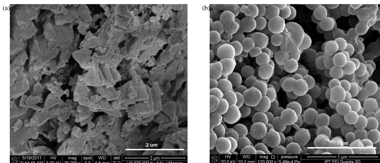
Fig. 9 Rifampicin micrographs obtained by SEM-FEG technique: (a) raw rifampicin without microfluidic process and (b) the rifampicin nanoparticles obtained in the reservoir device, using a flow rate of 2000  $\mu\text{L}/\text{min}$
