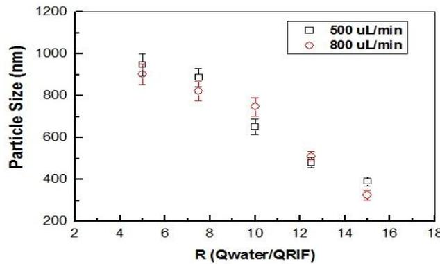
Fig. 5 Rifampicin particle size (nm) obtained in branching microfluidic device in terms of ratio between phases R ( $Q_{\text{water}}/Q_{\text{Rif}}$ ) for two different flow rates: 500 and 800  $\mu\text{L}/\text{min}$
