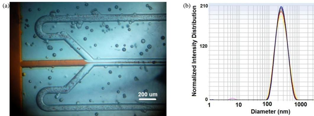
Fig. 4 Rifampicin flow focusing on reservoir microfluidic system: (a) detail of a flow focusing using ratio (R) between phases of 20 and a water flow of 2000  $\mu\text{L}/\text{min}$  and in (b) the rifampicin particle size measurement by DLS of 250 nm obtained in this flows conditions
