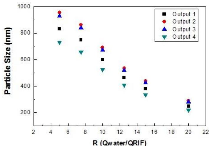
Fig. 7 Rifampicin particle size (nm) obtained in each output of reservoir microfluidic device in terms of ratio between phases R ( $Q_{\text{water}}/Q_{\text{Rif}}$ ) for a water flow rate of 2000  $\mu\text{L}/\text{min}$
