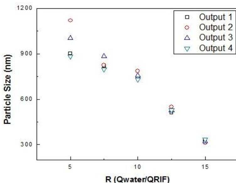
Fig. 8 Rifampicin particle size (nm) obtained in each output of branching microfluidic device in terms of ratio between phases R ( $Q_{\text{water}}/Q_{\text{Rif}}$ ) for a water flow rate of 800  $\mu\text{L}/\text{min}$
