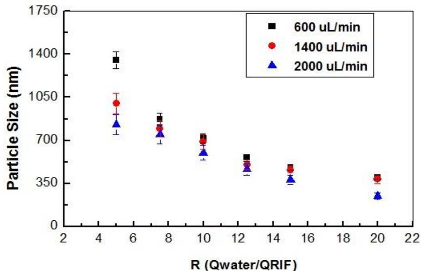
Fig. 3 Rifampicin particle size (nm) obtained in reservoir microfluidic device in terms of ratio between phases  $R$  ( $Q_{water}/Q_{Rif}$ ) for three different flow rates: 600, 1400 and 2000 μL/min
